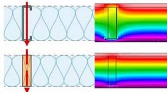
In the above cases, the studs are acting as thermal bridges for heat transfer.
